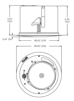
Figure 16. C6 loudspeaker dimensions
