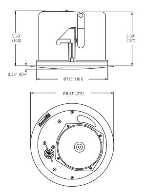
Figure 15. C4 loudspeaker dimensions
