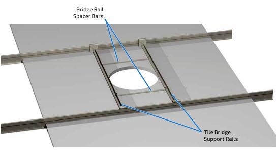
Figure 5. Tile bridge and spacer rail layout
