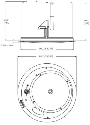
Figure 17. C8 loudspeaker dimensions
